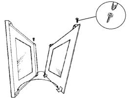
3 You should hold the door glass securely in place with one hand, whilst removing the screws completely, with the other hand. If you do not do this, the door glass could fall forward. Still holding the door glass, remove the trim from the top of the door.
